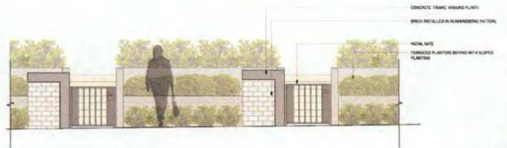
ELEVATION: PRIVATE STREET FACING ENTRIES SCALE 1:25
