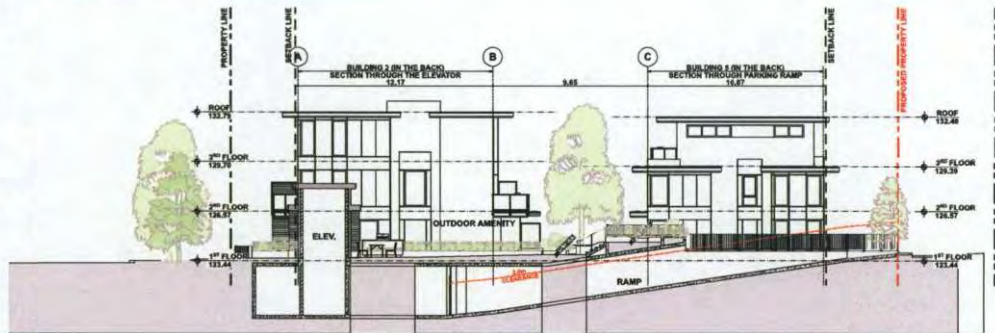
Section through mews and outdoor amenity - showing the change in grade
