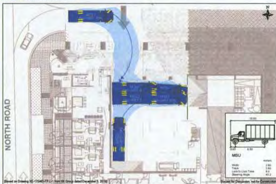
Exhibit 1a Type B Loading Space - Inbound Movement
