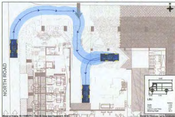
Exhibit 2a Type A Loading Space - Inbound Movement
