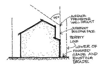
(iii) The *perimeter wall area* of each *outermost building face*, when considering the slope of the *lot*, will be determined by the following:
