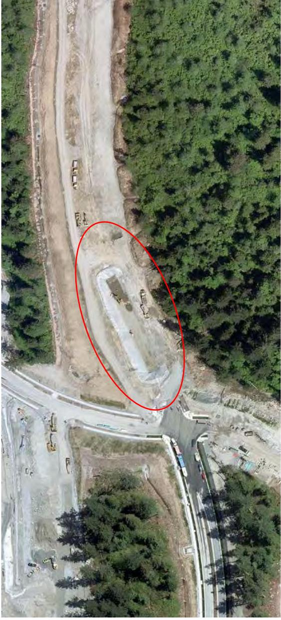
Inset B - 2017 aerial imagery illustrating construction of baseflow augmentation tank per Partington Creek IWMP.
