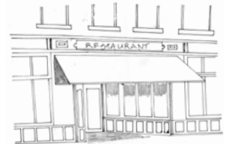
Demonstrates recessed commercial entrance, transom windows, awning, abundant windows and sign band
