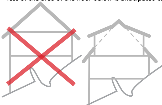
Discouraged: roof form added to 6th storey
