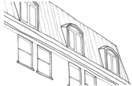
Demonstrates a contemporary mansard roof with dormers
