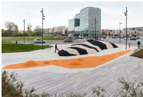
Fig.66 Example of recycled rubberized play surface
