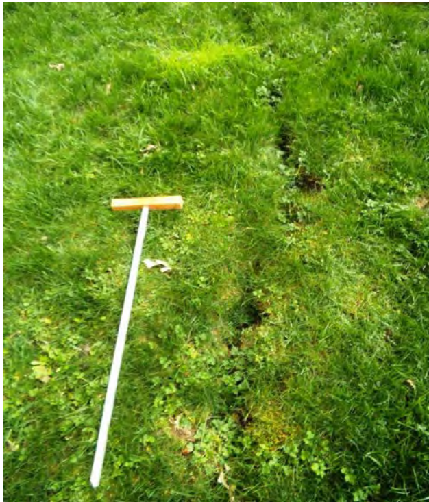
Tension crack or settlement feature, centre north half of back yard
