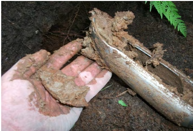
Downslope Soil Pit, With Wet Plastic Soil At Depth
