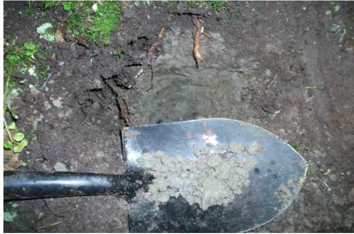
Soil Test Pit (in Fill?) Below Large Concrete Retaining Wall
