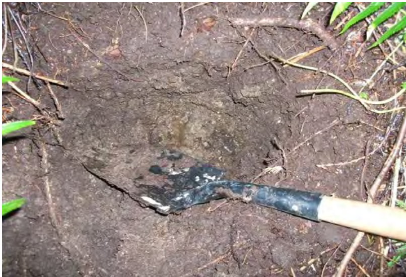
Shallow Soil Test Pit Below Crest Into Fill and Till, With Seepage
