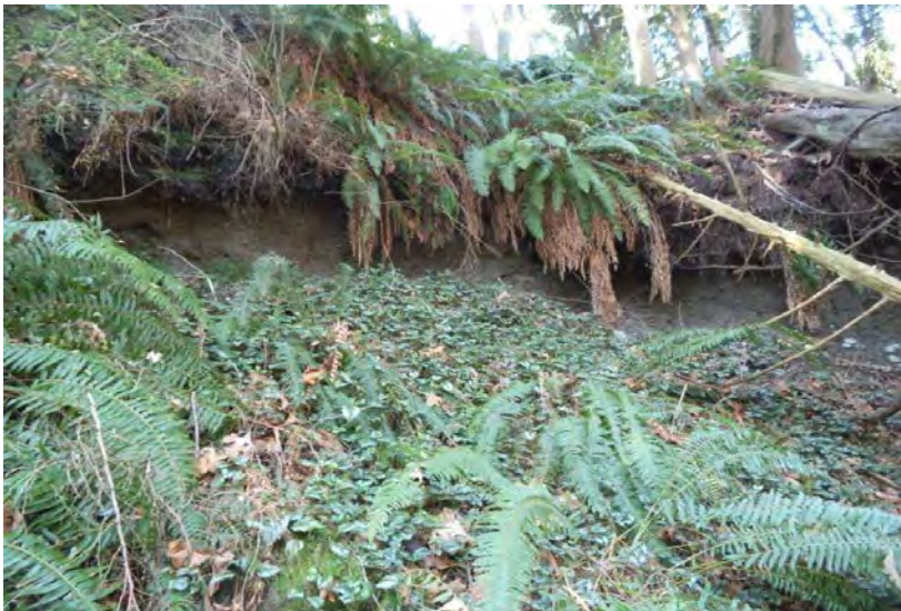
Headscarp of Failure Below Property Along Sundial Creek Tributary
