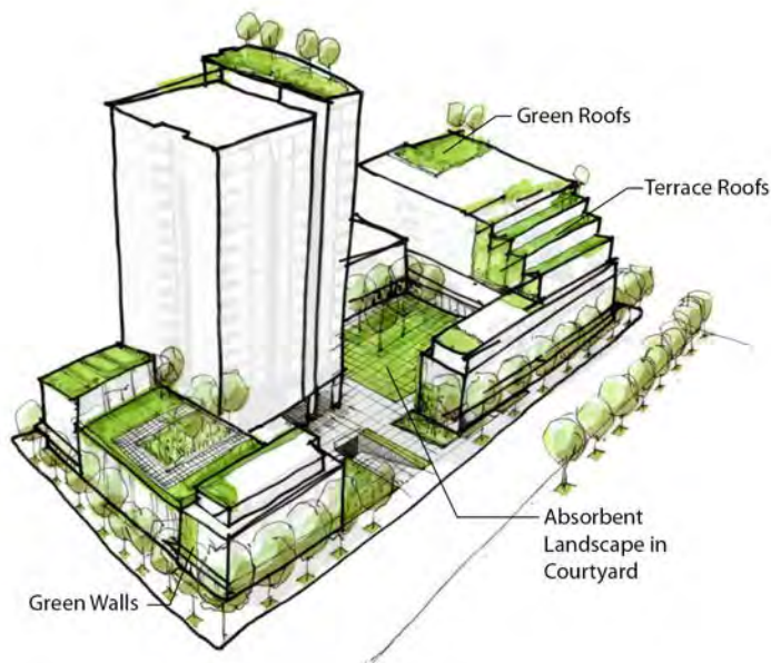
FIGURE 9-3 Onsite Rainwater Controls – Scenario 2
