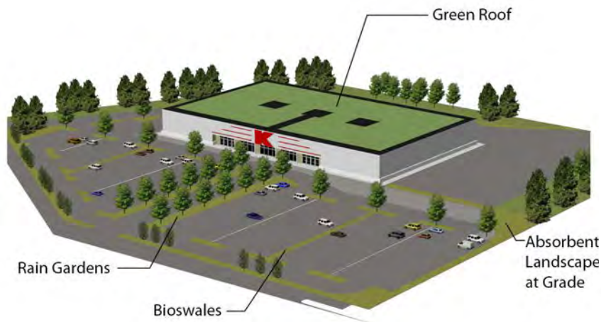
FIGURE 9-5 Large-format Retail Onsite Rainwater Controls
