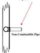
Notes; 1)Soil and waste stacks in walls are non-combustible cast iron and are sealed at each horizontal floor penetration with the appropriate S115 Fire Stop System. 2) Also see B.C.B.C. Article 9.10.9.7. as this is applicable in wood frame buildings
