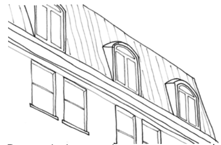
Demonstrates a contemporary mansard roof with dormers
