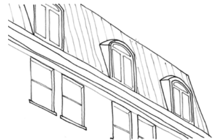
Demonstrates a contemporary mansard roof with dormers
