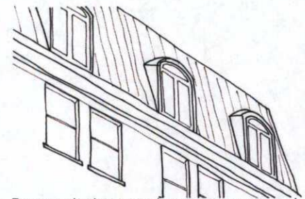
Demonstrates a contemporary mansard roof with dormers
