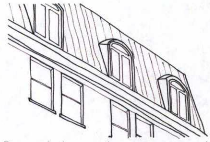
Demonstrates a contemporary mansard roof with dormers
