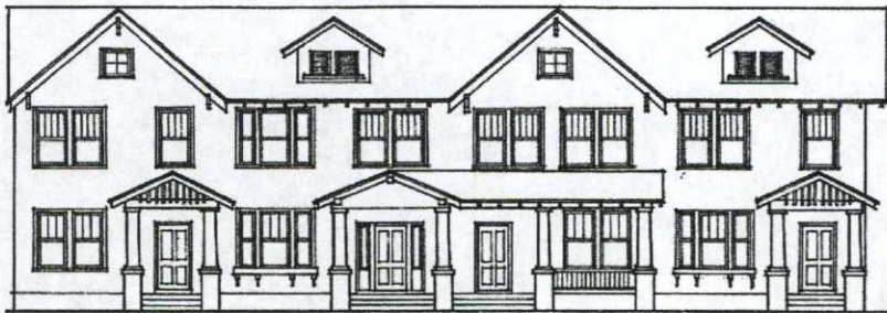
Demonstrates a consistent rhythm across the facade and vertical orientation of the windows
