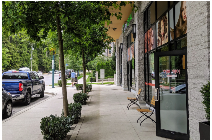
Space for door openings in Building Frontage Zone with landscaping to separate the space from the Pedestrian Movement Zone.
