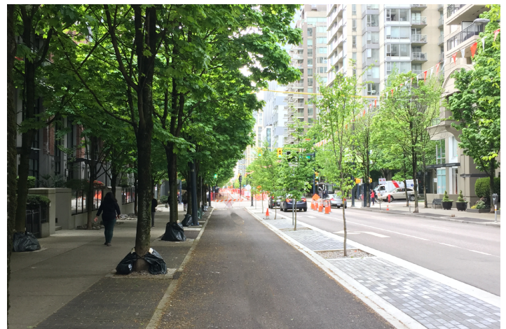
Micromobility Zone located between the Furnishing Zone and Buffer Zone with a combination of pavers and street trees.
