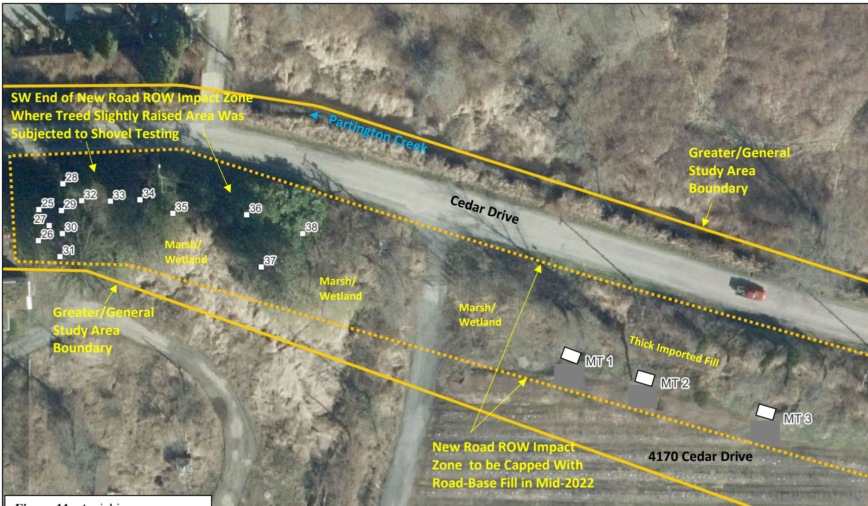
Figure 11. Aerial image map showing shovel test and machine test locations and new road ROW impact zone in Development Area 6 at the southwest end of the new road ROW at 4170 Cedar Drive. See also Figures 12 to 14.
