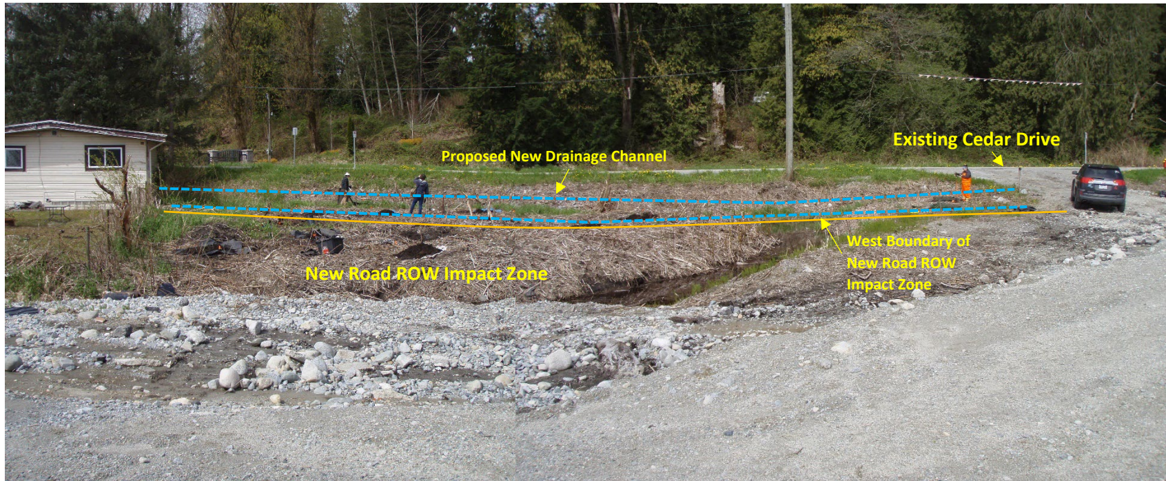
Figure 21. View of small area at the north end of 4169 Cedar Drive (left) and the south end of the road-base fill section of the ROW (right) with shovel testing in progress, looking west. Fifteen shovel tests (STs 53 to 67) were placed in this area, revealing that it is a former wet marshland that was built up by being capped with about 40 to 50 cm of imported fill containing a moderate quantity of domestic and industrial refuse. Note existing drainage ditch in the center of the photo. This location will be capped with road-base fill in mid-2022. See also Figure 15.
