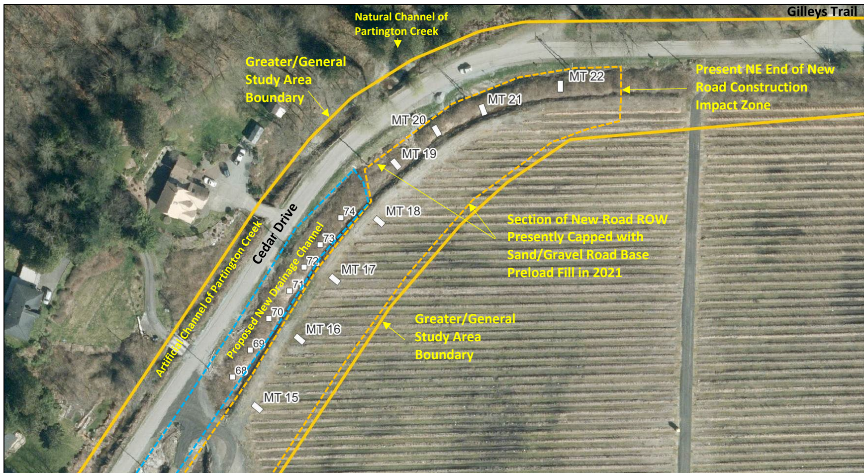
Figure 25. Aerial image map showing the NE section/end of the new road ROW in Development Area 7 that was capped with road-base pre-load in 2021 (not shown in photo), proposed drainage channel impact zone, Shovel Tests 68 to 74, and location of Machine Tests 4 to 14. See also Figures 29 and 30.
